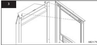
There are two flat clips supplied to grip the bottom edge of the front to the fire:
